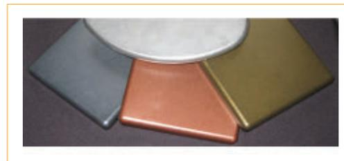
**Figure 3**—UV-cured powder coating metallic finishes on MDF.
